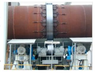
there are usually upper and lower "retaining (or thrust) rollers" bearing against the side of tyres, that prevent the
